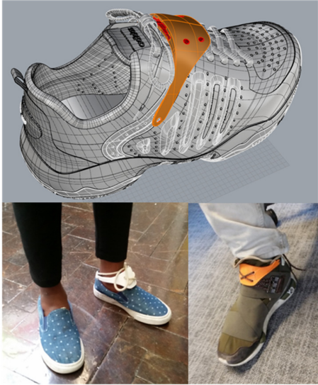
Figure 5: 3D printed show-flap protective shell for IMU
