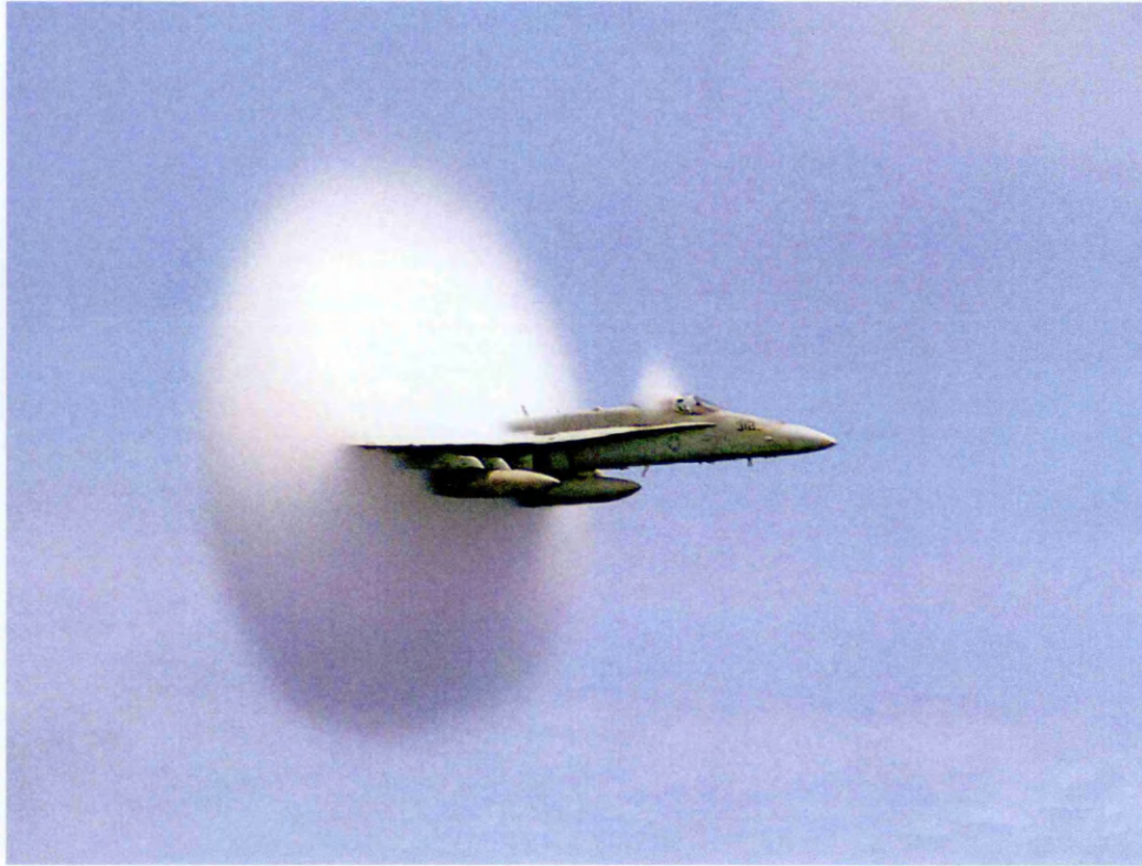
Figure 4.12: Clouds condensing behind the bow shock of an F/A-18 fighter jet as it accelerates to supersonic speeds. Image source/credit: NASA/Ensign John Gay, USS Constellation, U.S. Navy
