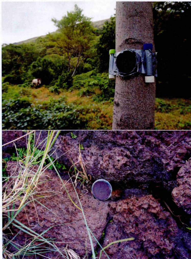
Figure 2.6: a) Photograph of SO 2 (purple) and acid gas (green) diffusion tubes and a sulfation plate attached to a tree. b) Photograph of a sulfation plate secured in a rock at ground level.
