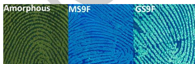
Figure 4. The three modes of visualization provided by the 9-fluorenone treatment. Left: non-crystalline or amorphous 9-fluorenone. Centre: metastable MS9F. Right: ground state GS9F. The pore locations within the fingerprint ridges are evident in each image. Images were visualized using a LUMATEC Superlite S04 forensic light source emitting 320–400 nm radiation and photographed with a Nikon D300 camera coupled with a DX Micro NIKKOR 40 mm Lens without filters.
