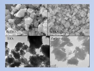
Microstructural changes due to mechanical activation in ZnO, BaTiO<sub>3</sub>, SrTiO<sub>3</sub> and TiO<sub>2</sub> powders were investigated using electron microscopy (TEM and SEM), x-ray diffraction (XRD) and particle size analysis (PSA). These were correlated with molecular simulations mechanical properties of **PVDF**nanocluster composites with different oxide nanocluster sizes (1, 1.5 and 2 nm)
