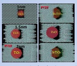
Each system was simulated using a periodic system of metal oxide nanocrystal inside β-PVDF matrix. β-PVDF was chosen for its superior properties over  $\alpha$ - and  $\gamma$ - phases. Geometry of each system was optimized prior to the calculation of mechanical properties using GULP v4.3 software package.
