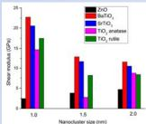
Molecular simulations show that, in general, mechanical properties (Young modulus as an indication of elasticity, Shear modulus as an indication of hardness) for all systems improve with decrease in nanocluster size. This suggests that mechanical activation of fillers in PVDF-metal oxide nanoparticle composites should have a positive effect on the mechanical properties of composite systems.
