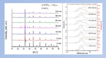
Mechanical activation leads to the creation of new surfaces and decrease in particle size of the powder particles, which affects the crystallization of PVDF matrix. In addition. mechanical activation leads prolonged agglomeration of nanoparticles agglomerates of different sizes.
