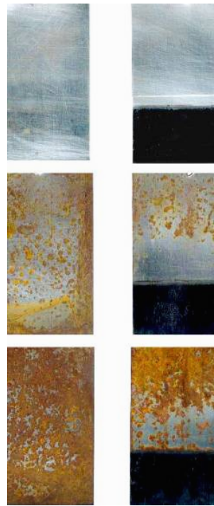
Figure 14. Images of the mild steel samples after one-day (top), 15-day (middle) and 45-day (bottom) exposure to atmospheric corrosion in Belgrade downtown. Left: bare mild steel, right: mild steel-PANI-benzoates.
