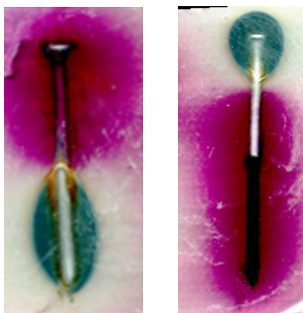
Figure 16. Ferroxyl indicator test of an unprotected (left) and a PANI-protected nail (right) after 10 h.
