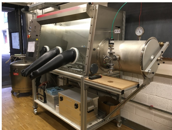
Figure 1: Glovebox with vacuum airlock for sample preparation
