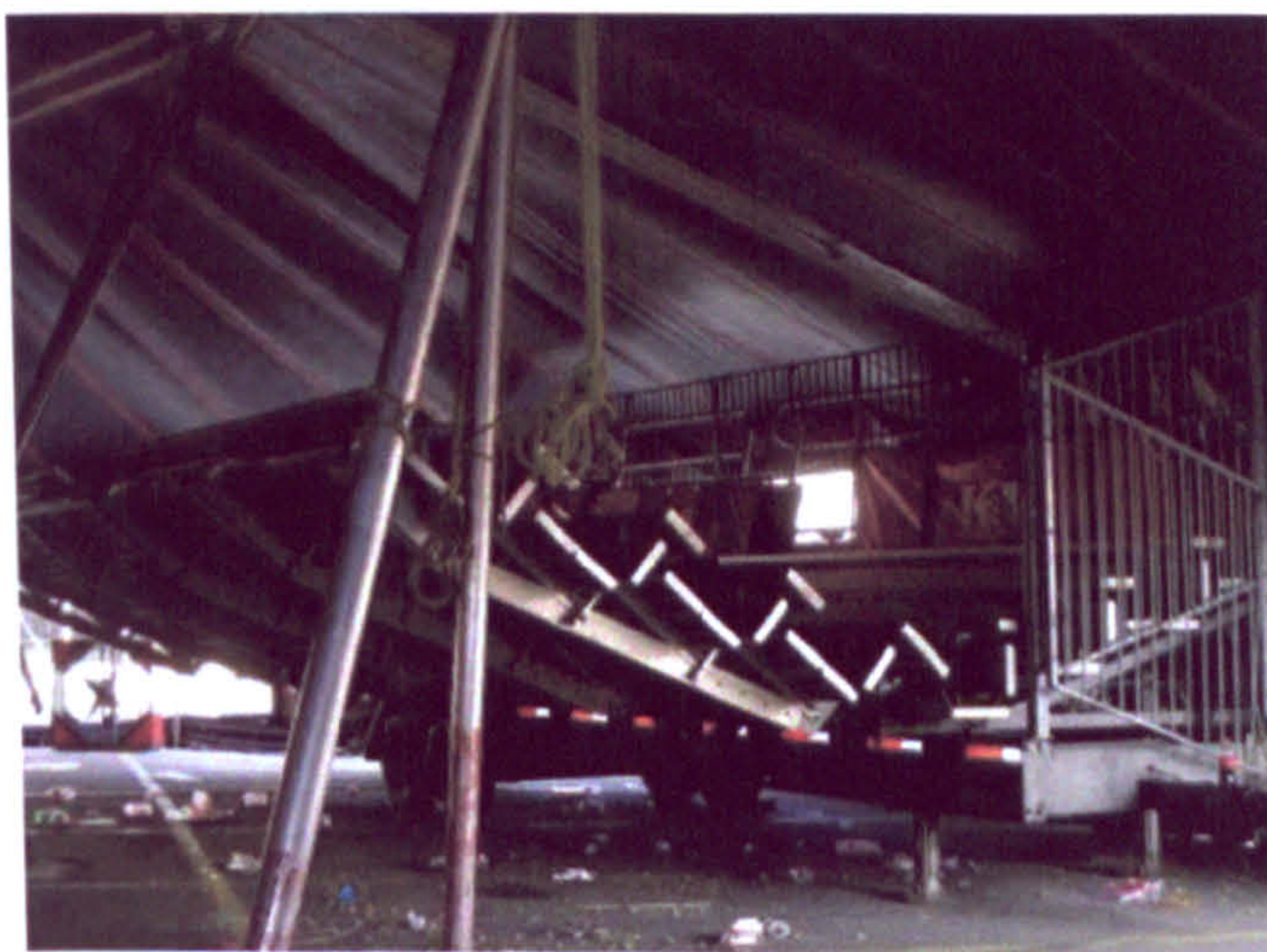
Figure 4.6: Greenville, PA on July 27. The bleachers fold up and secure the seating barriers for the drive.
