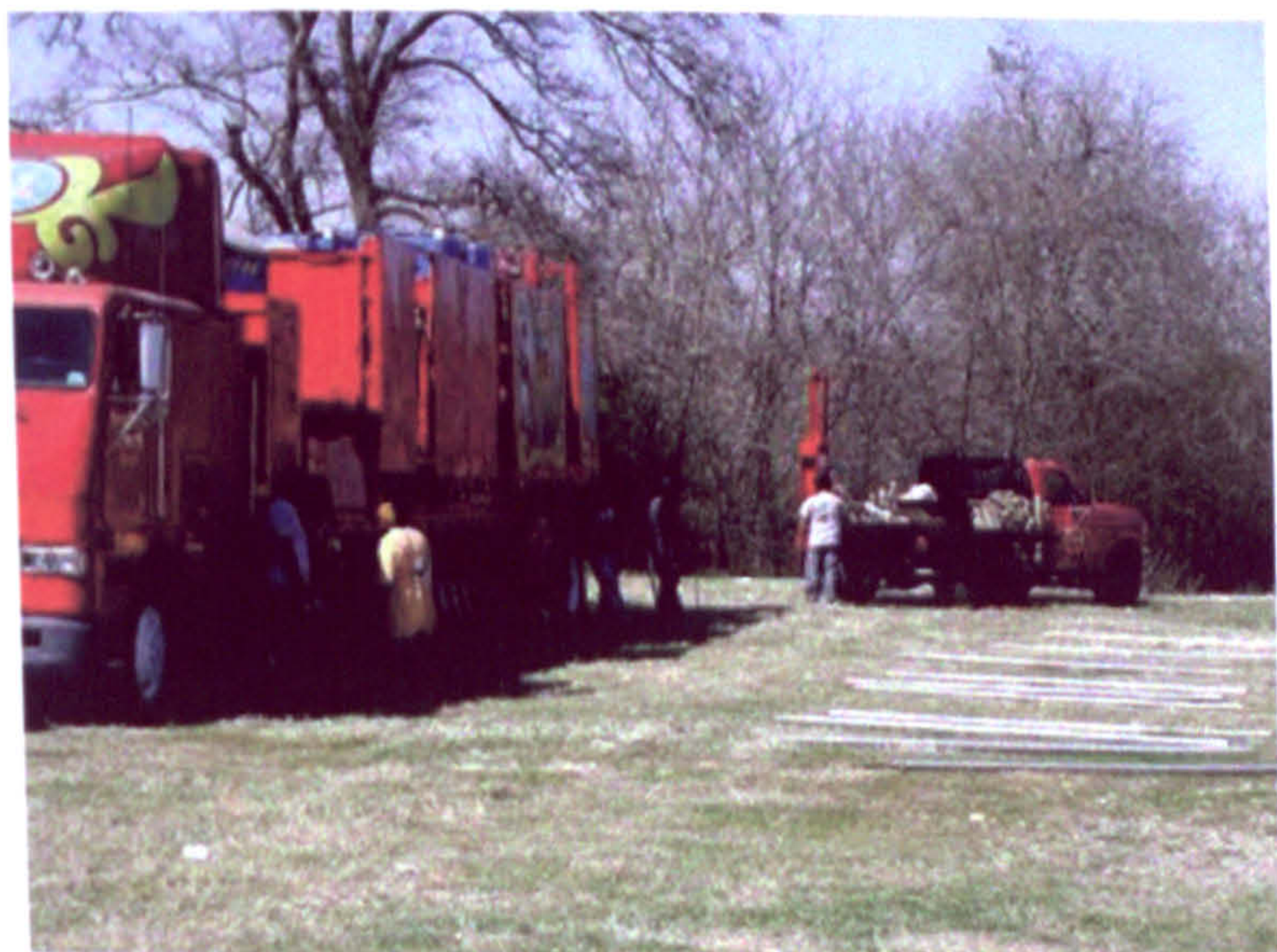
Figure 4.21: Hugo, OK on March 13. The mechanical stake driver pounds stakes around the circumference of the tent. This drive is considered when determining the layout of the lot.
