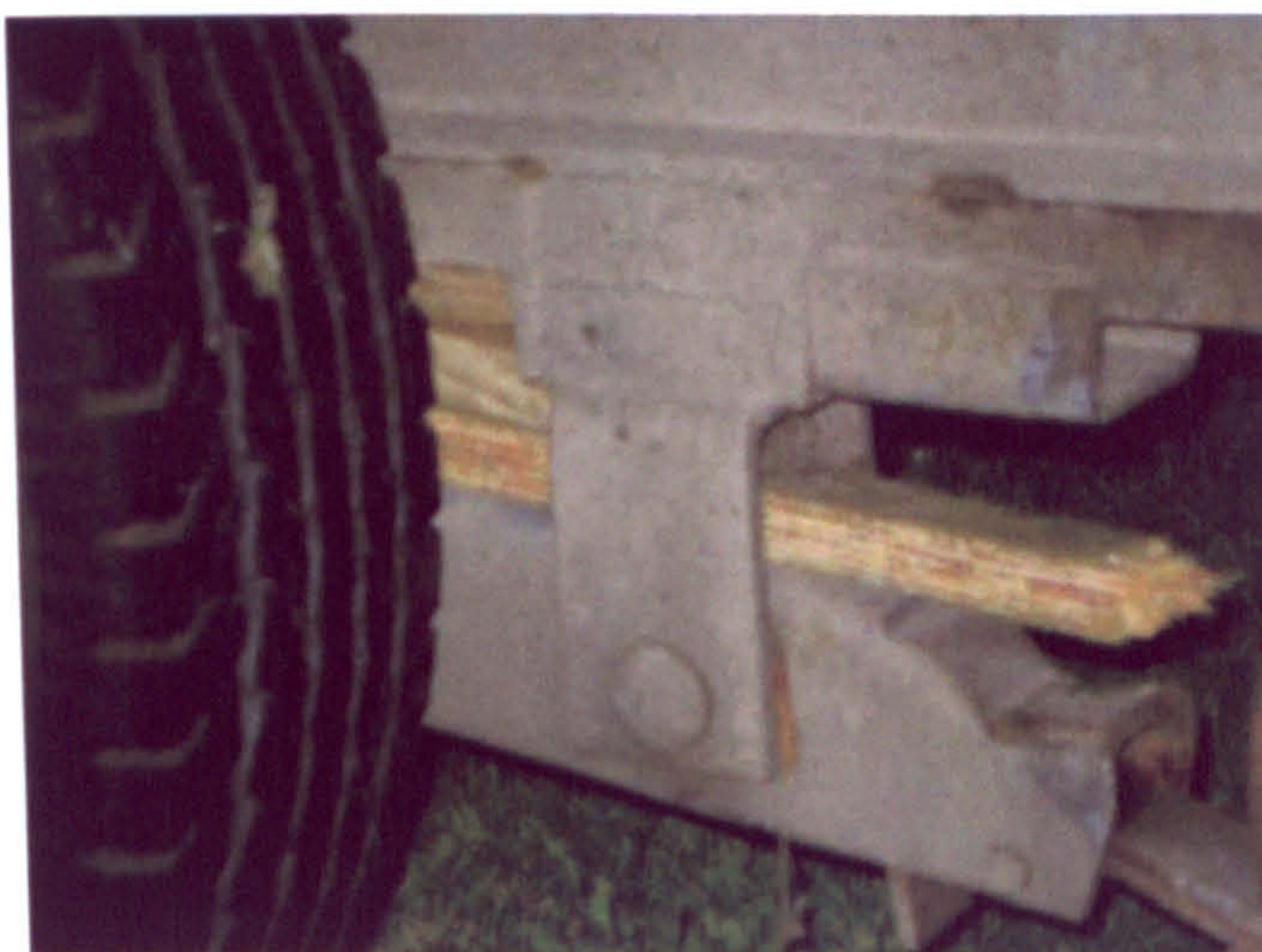
Figure 6.14: Kelly's Island, OH on August 5. A Circus Rigged truck suspension. This was one of the last photographs I took during fieldwork, right before the show pulled off the lot.
