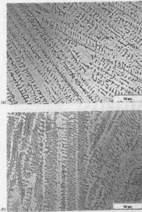
Fig. 2.24 Fusion zone microstructure resulting from mode FA solidification: (a) skeletal ferrite; (b) lathy morphology [90].
