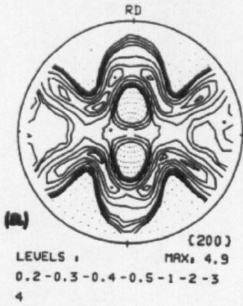
Fig. 1.30 {200} pole figure of cold rolled copper, 50 \mu\text{m} , cold rolled 95% [49].
