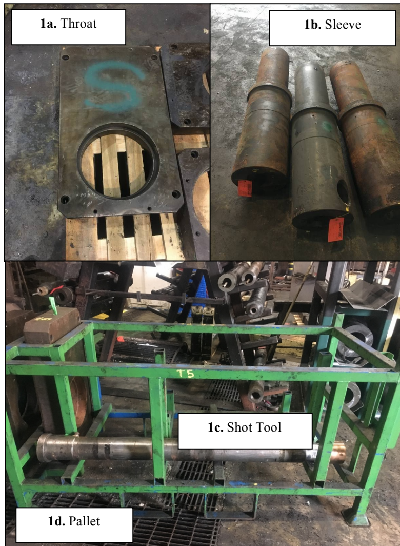
FIGURE 1: Throat, Sleeve, Pallet and Shot End components.
