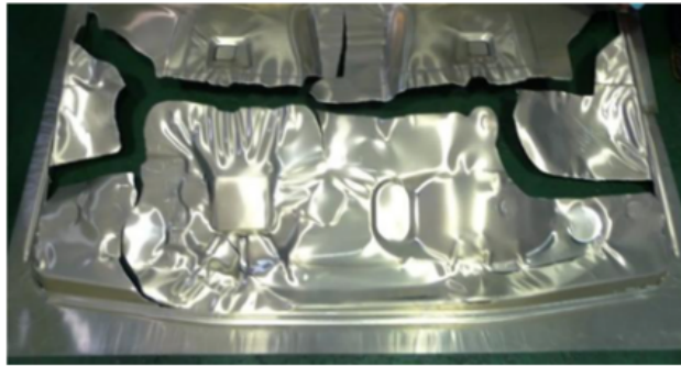
FIGURE 6: Ruptured product of the dash panel (Park and Kwon, 2015).
