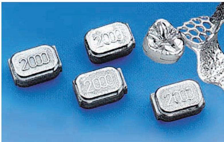
Fig. Alloy "Remanium – 2000" (Germany) for manufacturing of arch prosthesis frames
