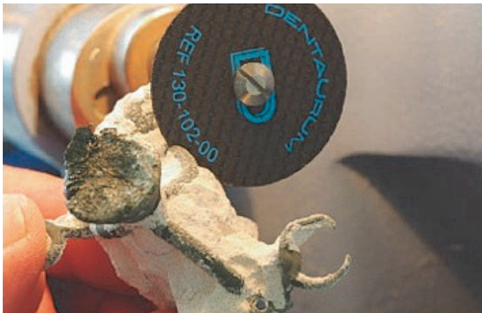
Fig. Cleaning of the cast frame from the fragments of forming masses
