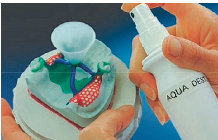
Fig. Preparation of wax composition on porcelain refractory model for making casting form
