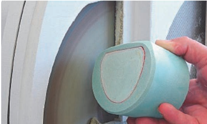
Fig. Formation of the required shape for the refractory mold before metal pouring
