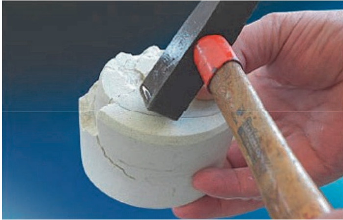
Fig. The release of the metal frame from the forming mass
