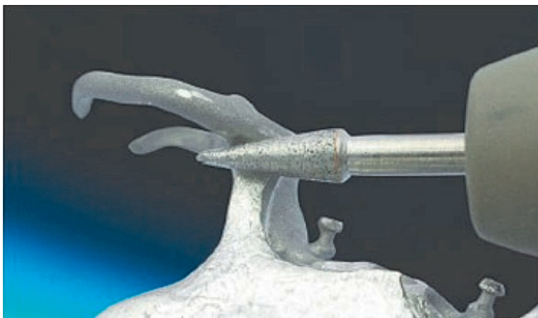
Fig. Grinding of the arch prosthesis frame in the clasp area
