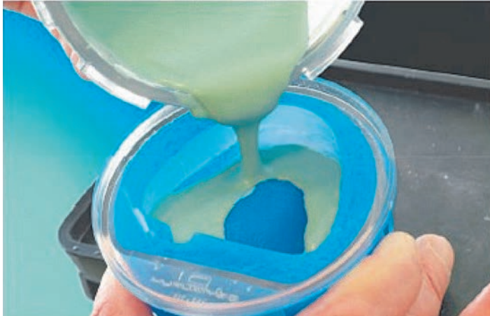
Fig. Filling of duplicating form by porcelain refractory mass
