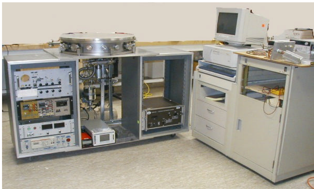
Fig. 2.3. The charge storage chamber and integral equipment rack with computer control.
