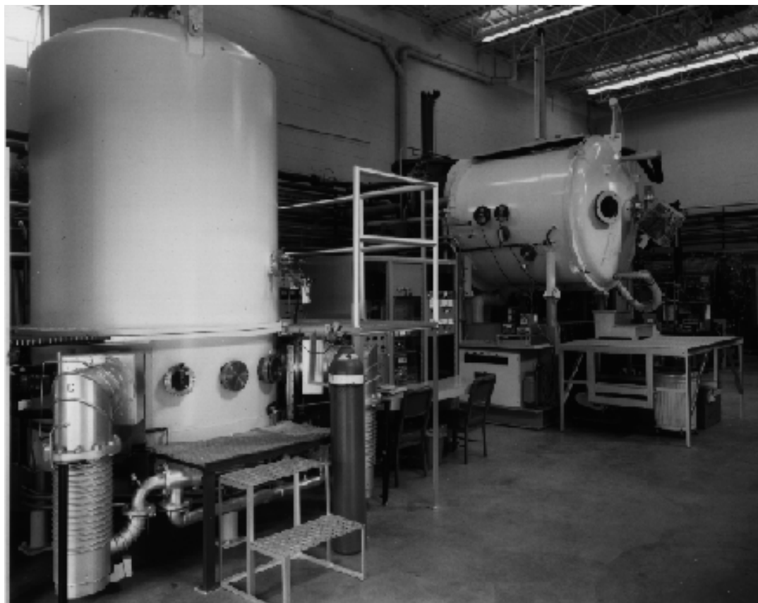
FIG. 3.3. NASA GRC Plasma Interaction Facility (PIF) (NASA Space and Environment Effects Branch Web Site, 2001). Of the two large plasma chambers shown, our experiments were performed in the chamber on the left.
