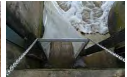
Filtering system for overflowing water. The system was checked every 15 minutes during overflow periods. © P. Baran
