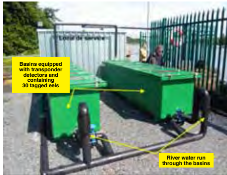
The MIGROMAT® system set up on the Killaloe site in Ireland. © F. Travade, EDF
