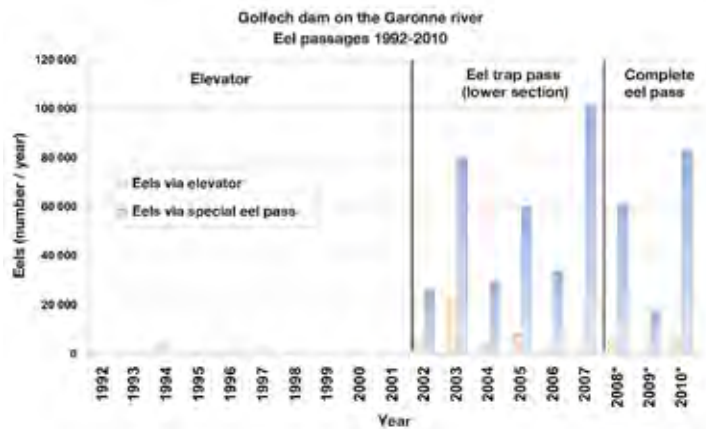
Number of eels passing the EDF Golfech hydroelectric plant on the Garonne river from 1992 to 2010. 1992-2001: Fish elevator alone. 2002-2007: Addition of a special trap pass for eels with manual transfer to the top. 2008-2010: Completion of the special fish pass for eels.
