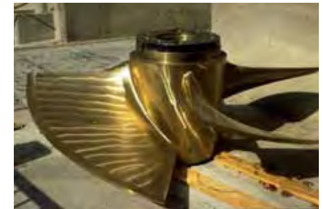
Runner of a three-blade Kaplan turbine. © M. Larinier
