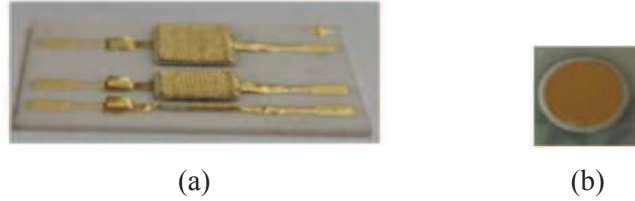
Figure 1: Photograph of a) piezoelectric bridges ( 5 \times 3.3 \times 0.08 \text{ mm}^3 , 3.3 \times 3.3 \times 0.08 \text{ mm}^3 , 3.3 \times 1 \times 0.08 \text{ mm}^3 ) and b) straightforward electroded microceramic ( \varnothing 9.5 \text{ mm} , thick. 190 \mu m)
