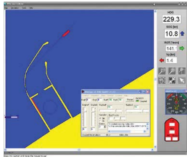
Figure 5. Interface depicting simulation model Design turning at outer turning points S (left) and B (right) in Mielno port (limited task simulator).
