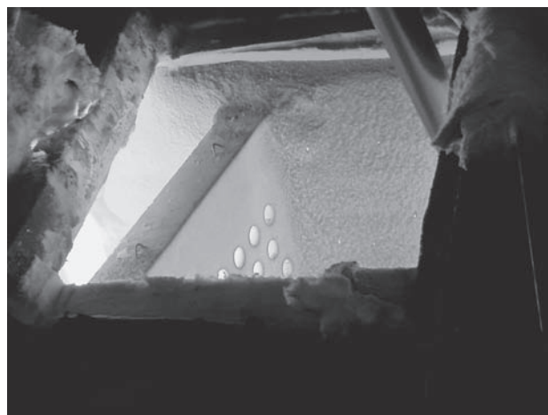
Figure 1 Tundish of the CC machine provided with the ceramic filter
