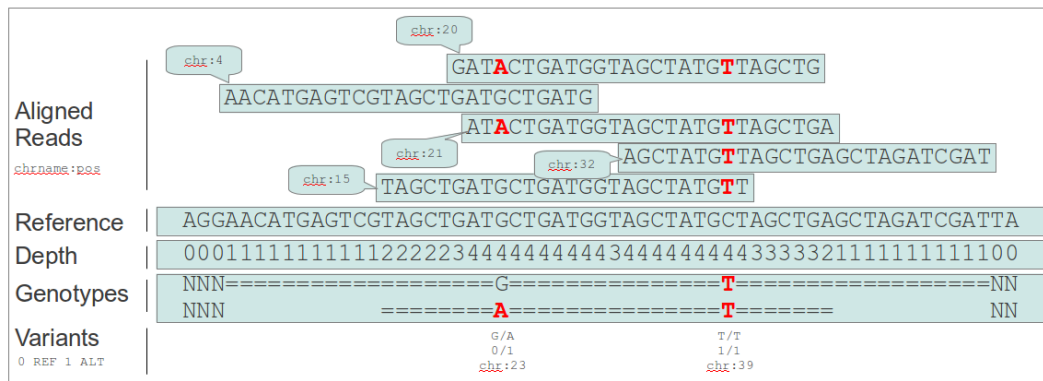
Figure 4.2: Representation of alignment. Reads are compared to a reference genome. When matching they are assigned a positional label. A locus depth is how many reads do actually support its genotype call. A naive genotype call is shown, in the real case complex quality considerations are performed before assigning a genotype. When read depth is zero, no genotype could be called. When just one, no diploid genotype could be confirmed.
