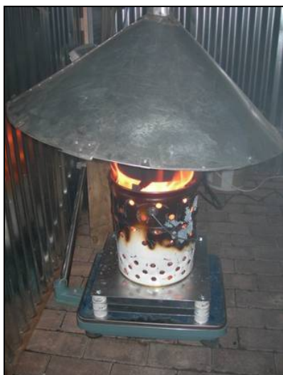
Figure 2. A typical imbaula on a test rig
