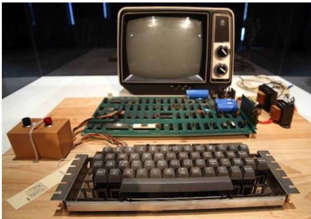
Fig. 3. A view of Apple 1 consisting in a motherboard connected with a keyboard and a domestic TV apparatus
