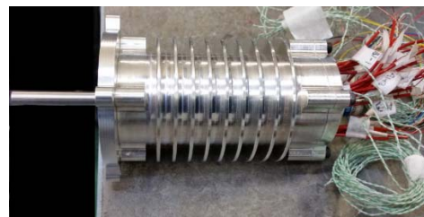
Fig. 3. PMSM driving the landing gear EMA.
