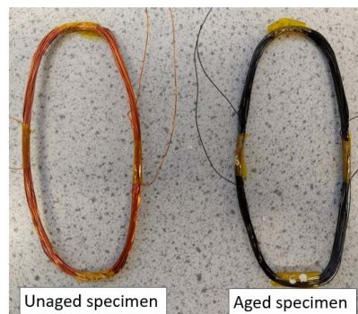
Fig. 14. Comparison between unaged (left) and thermally aged (right) specimens.
