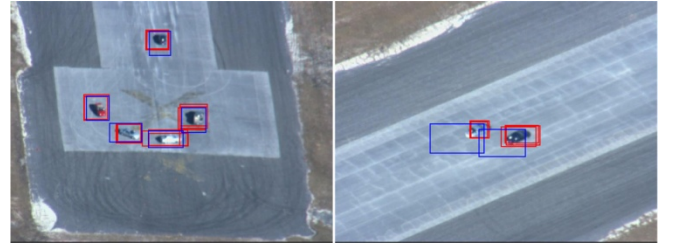
Fig. 2. Segmentation results of FMHI and prediction. The FMHI results are marked by rectangles with blue color, and the results obtained by prediction are marked by rectangles with red color.
