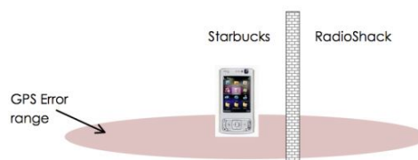
Figure 19: Localization error caused by a dividing wall [5]
