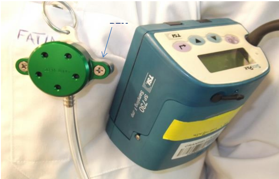
Plate A-6 Collection of airborne particles with PEM with using sidepak pump
