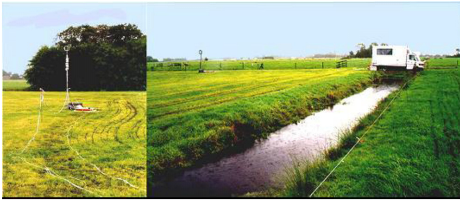
Figure 7. Eddy covariance flux measurements at Zegveld (NL) over a manured field. Left: mast with an ultra-sonic anemometer and sample inlet line. Right: the sample line is connected to a TDL housed inside the electrically powered mobile laboratory.
