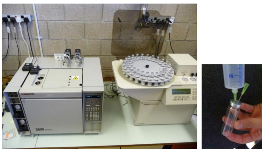
Figure 2. The left picture is an example of a typical GC fitted with an electron capture detector for N 2 O analysis and a flame ionization detector for CH 4 and CO 2 analysis (left) linked to an autosampler containing the sample vials. Gas samples are usually collected by syringe and stored in either pre-evacuated vials or, as shown in the right picture, by flushing a large sample volume through a small vial. As N 2 O is a stable gas vials can be stored for several weeks before analysis.
