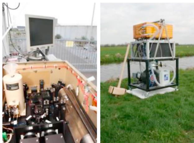
Figure 3. Infrared \text{N}_2\text{O} sensors are robust field instruments. This Quantum Cascade Laser spectrometer for \text{CH}_4 , \text{N}_2\text{O} and \text{NH}_3 (Aerodyne Instruments, Massachusetts) is deployed in an intensively managed grasslands (NL).
