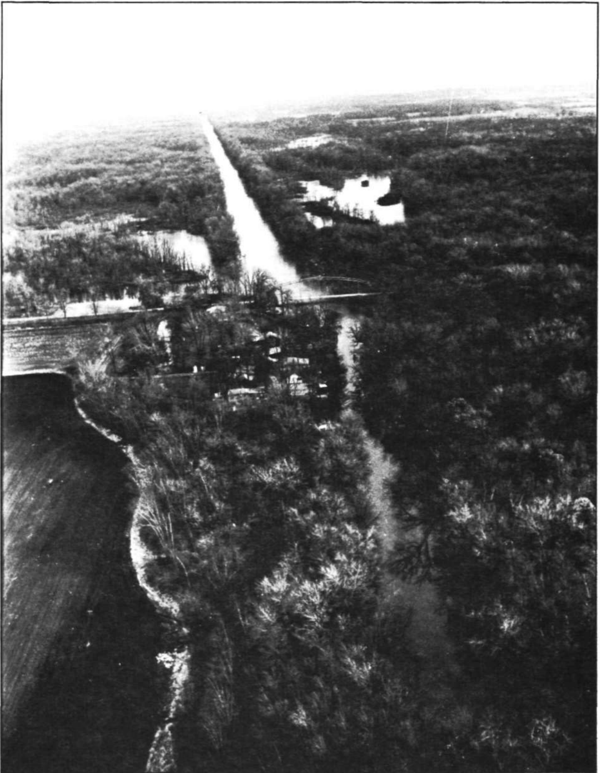
The Kankakee River at the Illinois-Indiana state line. The bridge is on the state line. The channelized portion of the river in Indiana is shown in the background and the naturally meandering portion of the river in Illinois is shown in the foreground. (Chicago Tribune photo)
