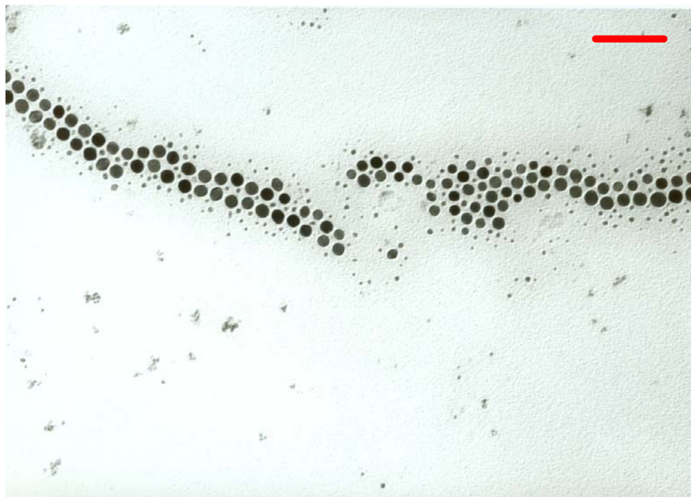
Figure 2.5: TEM image of cobalt nanoparticles ( 19.7 \pm 2.8 nm) prepared from oleic acid and TOPO. Bar= 100 nm
