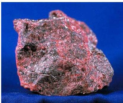
Figure 1. Cinnabar, the principal ore of mercury (Andel, 23/12/13 via Wikimedia Commons, Creative Commons Attribution)
