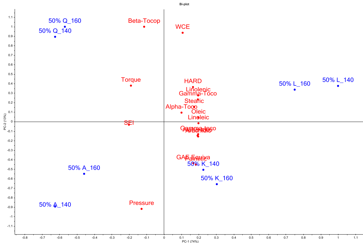
Figure 14b. PCA-biplot on the extrudates processed at 50% content of tested flour at two different extrusion temperature conditions (140 and 160 °C) (Temp-Temperature, TOR-Torque, SEI-Single expansion index, WCE-water content of extrudates, PRE-pressure, HARD-Hardness, A-Amaranth, Q-Quinoa, K-Kañiwa, L-Lupine). R^2Y for the first component was 74% and the difference between the first and second principal component was 13%.
