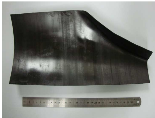
Fig. 11 An anisotropic composite tooling by ACT design
