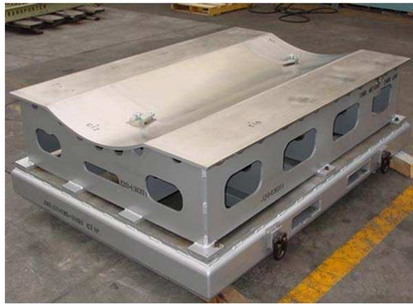
Fig. 6 Lockheed F-35 Invar laminating tooling [25]
