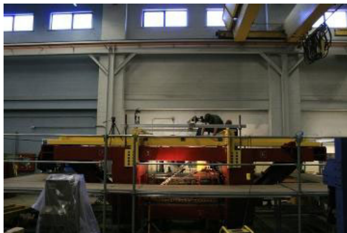
Figure 1. Full-scale steel grillage experimental setup.
