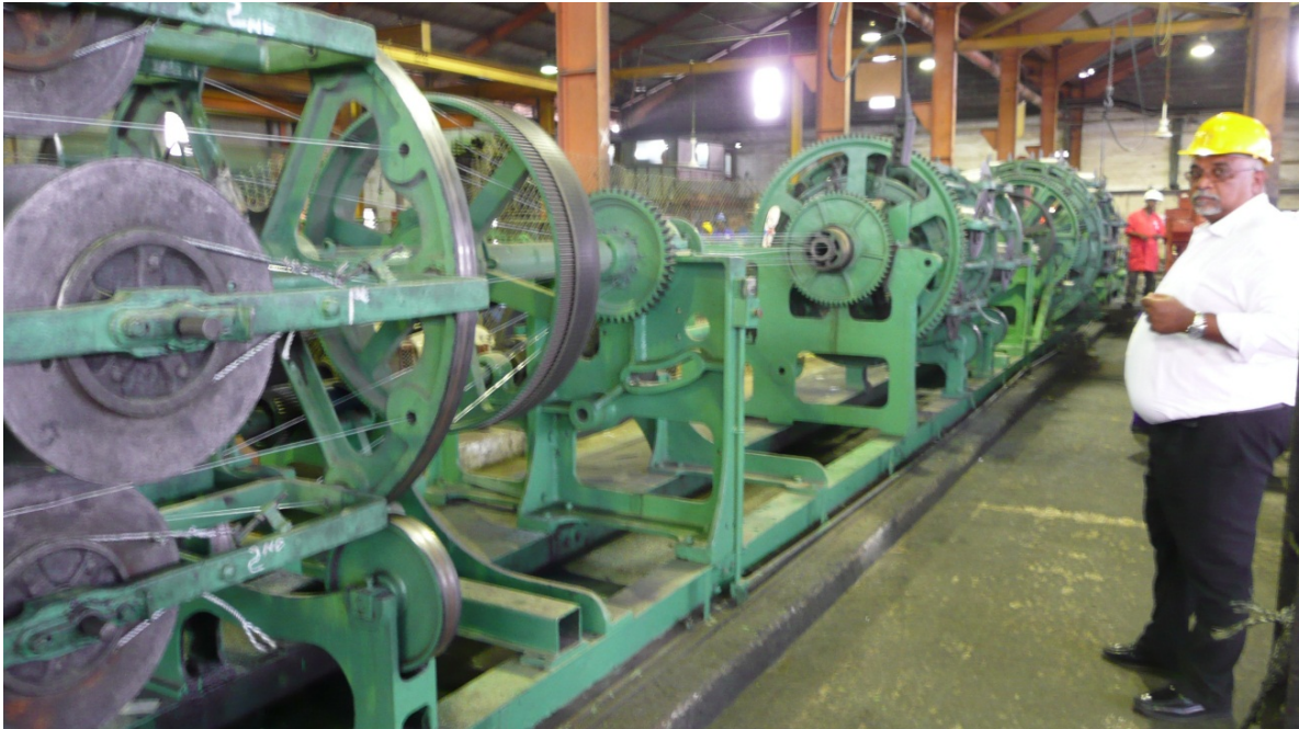
Figure 5.6 Steel cable production line in the Nigerian Ropes factory. Source: author.
