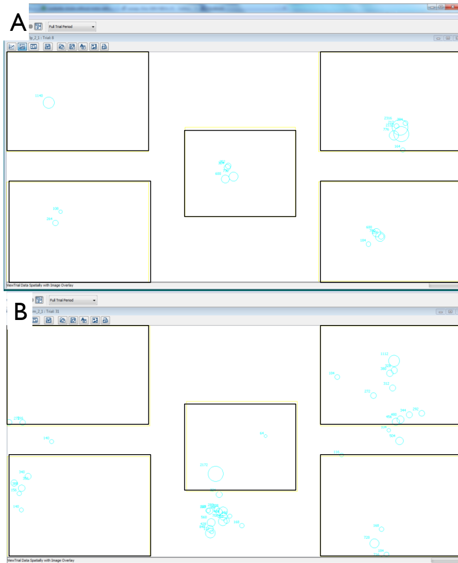
Figure 1. Fixation record of a visual world trial. Fixations indicated in cyan, interest areas in yellow (overlaid with black for clarity) A. A typical trial; fixations largely fall into the interest areas, no systematic deviations. From the fixation density, it is clear that the target was in the upper right-hand corner. B. In this trial, fixations are systematically lower than the interest areas, indicating calibration problems. Here the target is in the upper right-hand corner, which means no target fixations have been lost. The fixation record was moved up.
