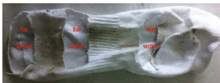
Fig. 2. Sectioning of sample for sock malodour study.
