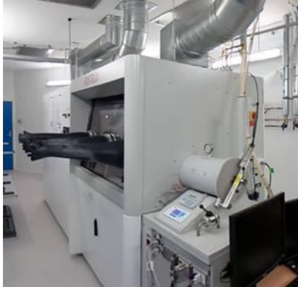
Figure 2.1: Photograph of the AIXTRON MOCVD reactor used in this work for growth of GaN and InGaN/GaN MQW structures.
