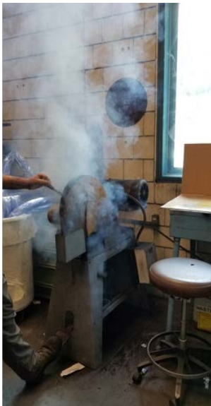
Figure B1. Smoke plume produced from cutting wire-reinforced hose surrounds a worker. There is a ventilation fan in the ceiling that is drawing smoke slowly away. Photo by NIOSH.
