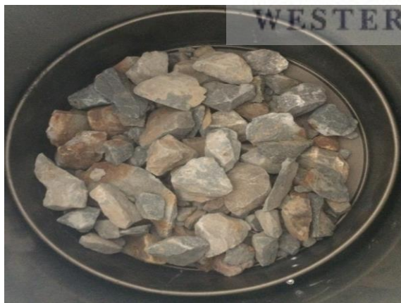
Figure 5.17 The uranium bearing sandstone, roughly 2kg, was placed in the chamber to measure the radon exhalation with the RAD7.
