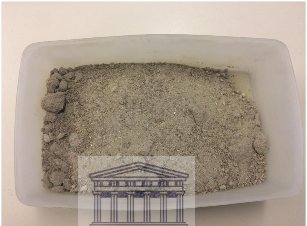
Figure 5.5 Philippi sand. about 2kg, placed in a pan before it was placed in the chamber to measure the radon exhalation with the RAD7.
