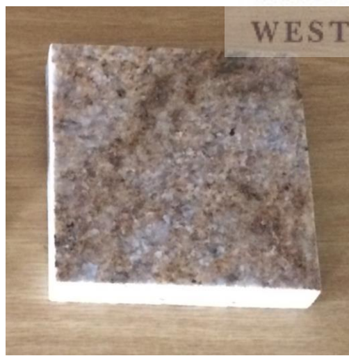
Figure 5.20 The Golden beach granite used for measurements using the RAD7 and HPGe.
