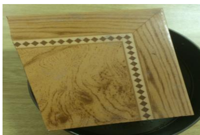
Figure 5.9 The floor tile, with mass of 650,4g, was placed in the chamber to measure the radon exhalation.
