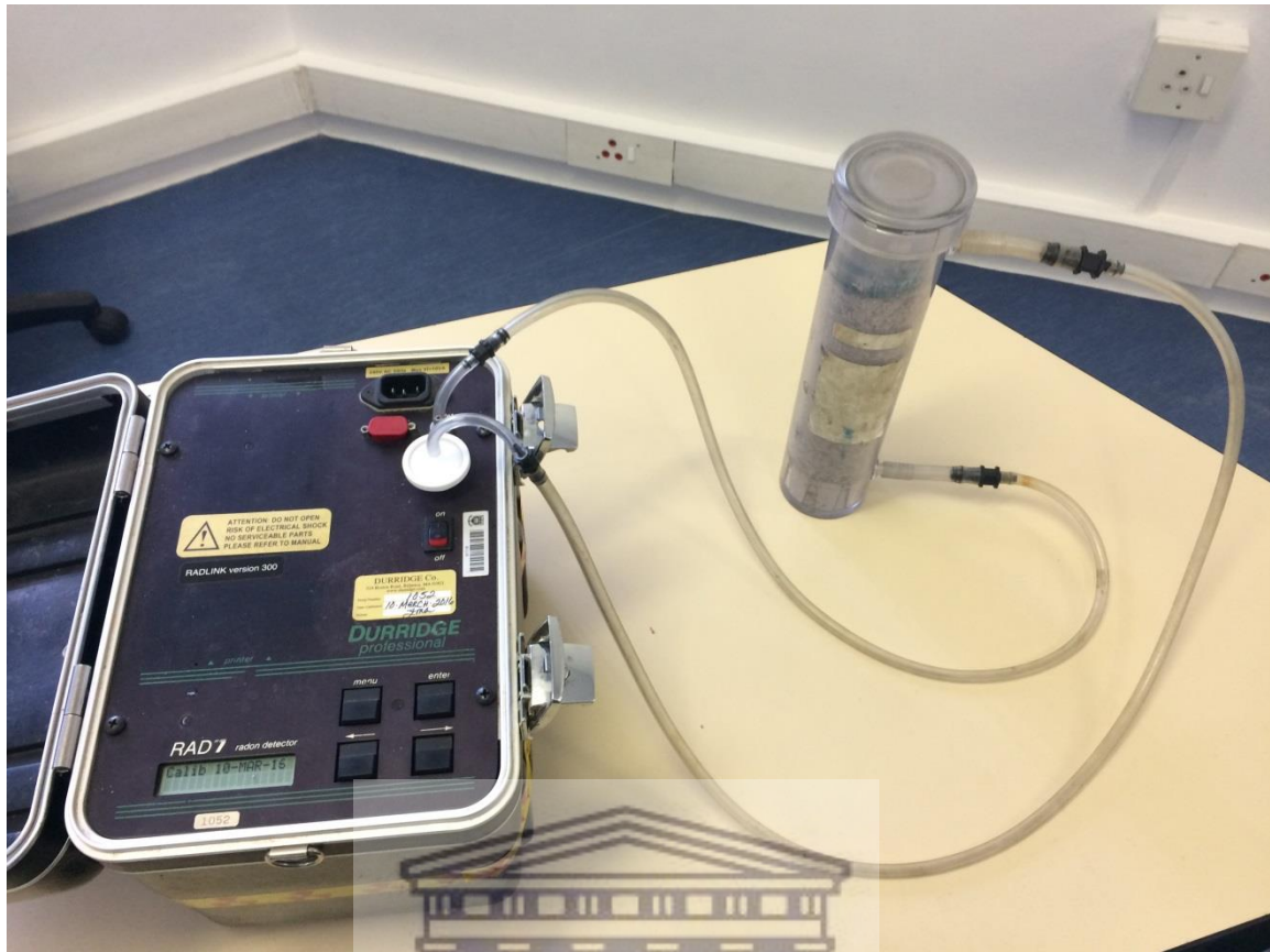
Figure 4.4 Purging taking place to reduce the relative humidity inside the RAD7.
