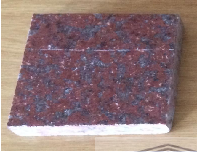
Figure 5.28 The African Red granite used for measurements using the RAD7 and HPGe.
