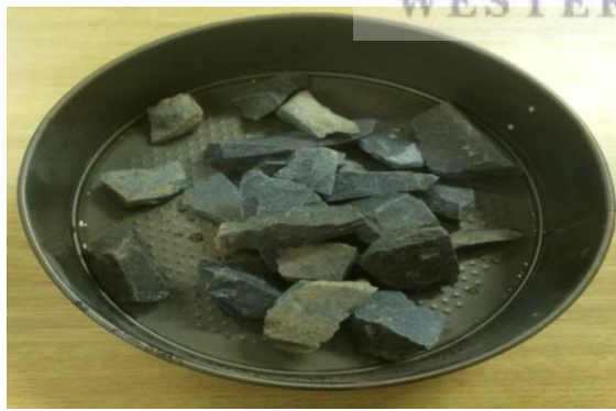
Figure 5.13 The Hornfels stones, with mass of 680 grams, were placed in the chamber to measure the radon exhalation.
