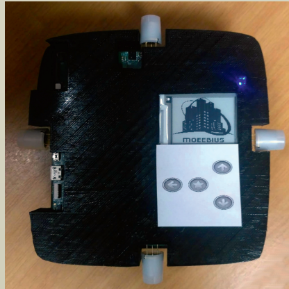
MOEEBIUS-NOD, a wireless multi-sensor device.
