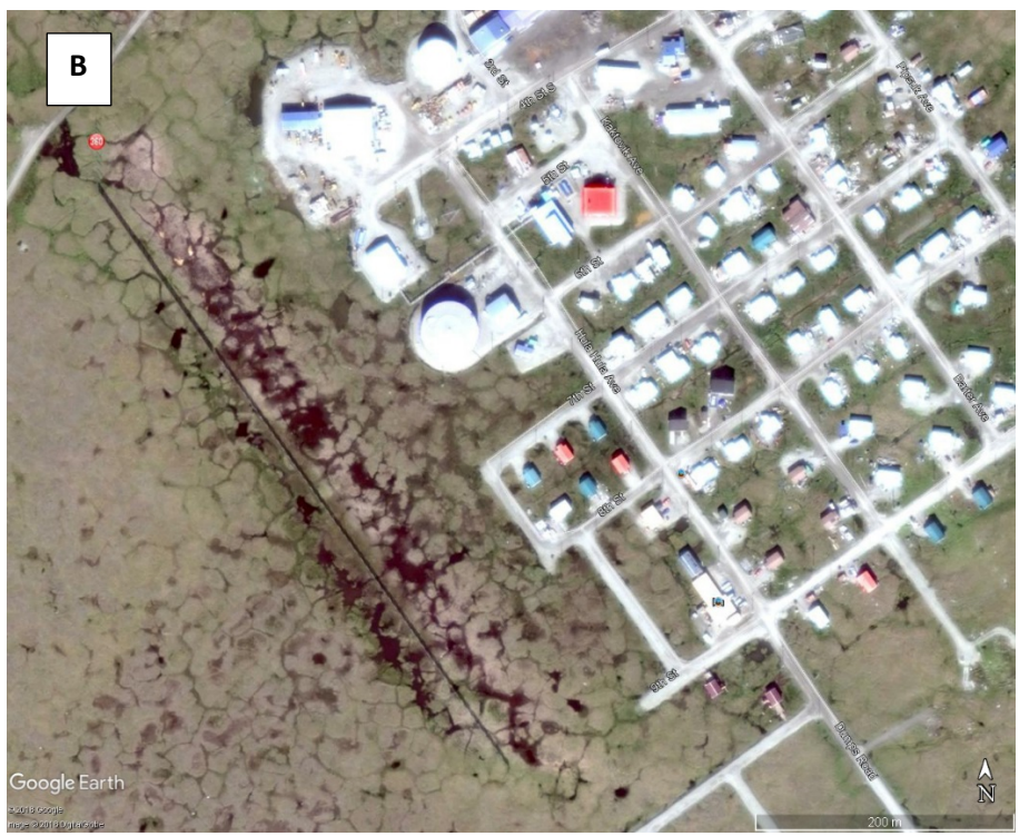
Figure 8. Thermokarst ponds developed as a result of ice-wedge degradation caused by (A) accumulation of surface water near embankment (Utqiagvik airport), and (B) accumulation of snow around snow fences (Kaktovik).
