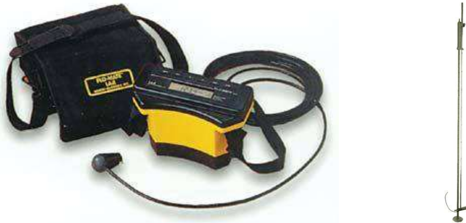
Figure 6. Marsh-McBirney Flo-Mate Model 200 Portable Flowmeter and Rickly USGS Top Setting Wading Rod
