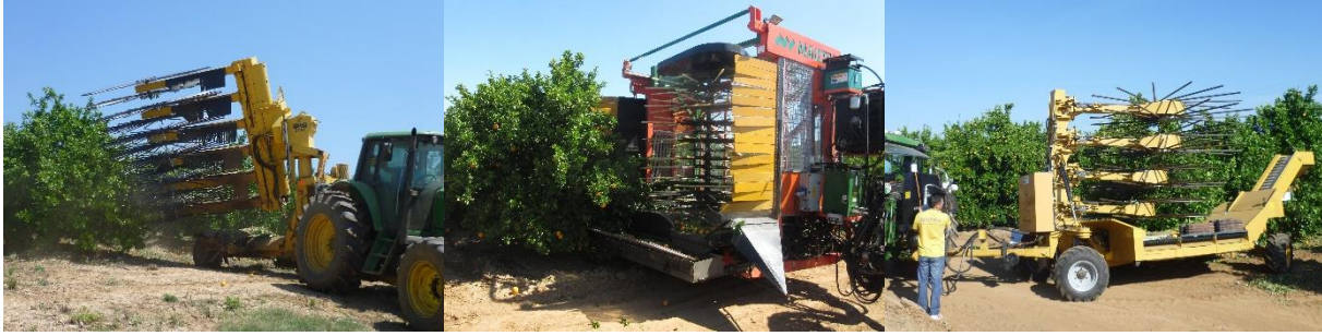
Figure 1. Tractor-drawn continuous canopy shaker systems used in citrus harvesting tests. Left: CS-1: Oxbo,3210; Centre: CS-2: Mediolive Prototype; Right: CS-3: Samolive Prototype.
