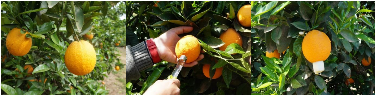
Figure 2. Placement of the acceleration sensor inside an orange before mechanical harvesting.
