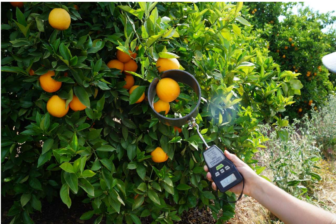
Figure 2. Measurement of citrus fruit detachment force with a pull test.
