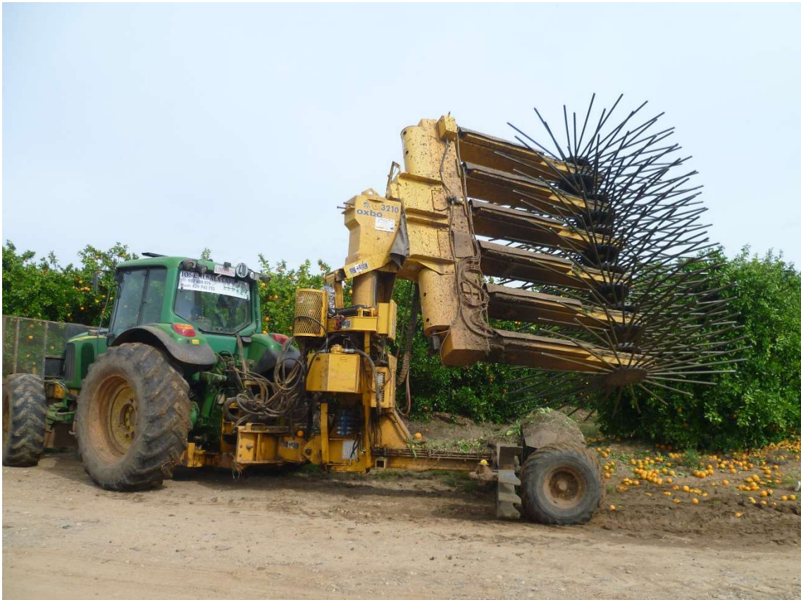
Figure 1. Mechanical citrus harvesting with a tractor-drawn continuous canopy shaker system (Oxbo, 3210).
