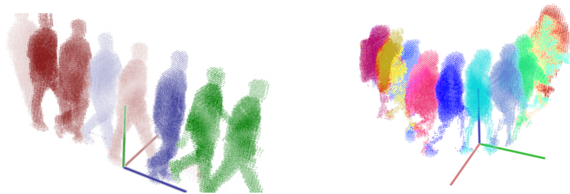
Fig. 4: 3D reconstructed gait sequences. Example of reconstructed gait sequences, sampled at 2Hz, where each point represents the center of a squared voxel.
