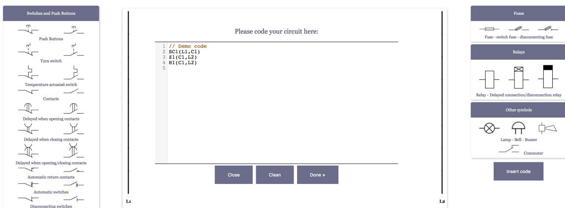
Figure 7. Example of the code for a basic electrical diagram. It is composed of a switch that activates a relay turning on a lamp.
