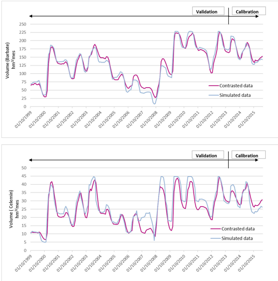
Figure 5: Comparison of contrasted values (fuchsia) and simulated (blue) for the calibration and validation of the model. Above: volume dammed at Barbate. Below: volume dammed in Celemín.
