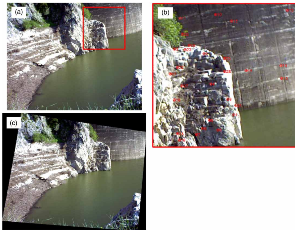
Figure 7 | Example of processed time-lapse photography: photo taken on 24/04/2013 in location 1 (near the dam): (a) original image, indicating the area geometrically adjusted by control points, (b) detail of control points considered, (c) geometrically transformed image.
