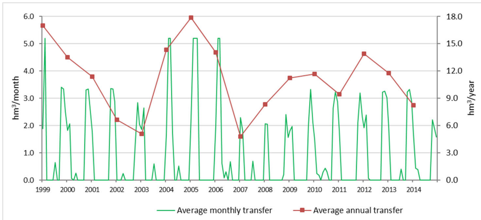
Figure 11: Monthly and annual average flows transferred between Barbate and Celemín reservoirs in the proposed strategy (E5a).
