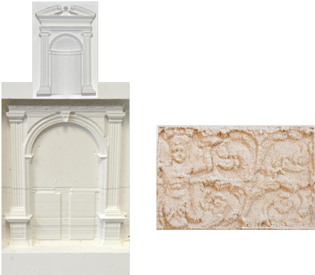
Figure 39. Image of two physical reproductions of the Portal made by numerical control milling. On the left: on plaster, and on the right: on wood
