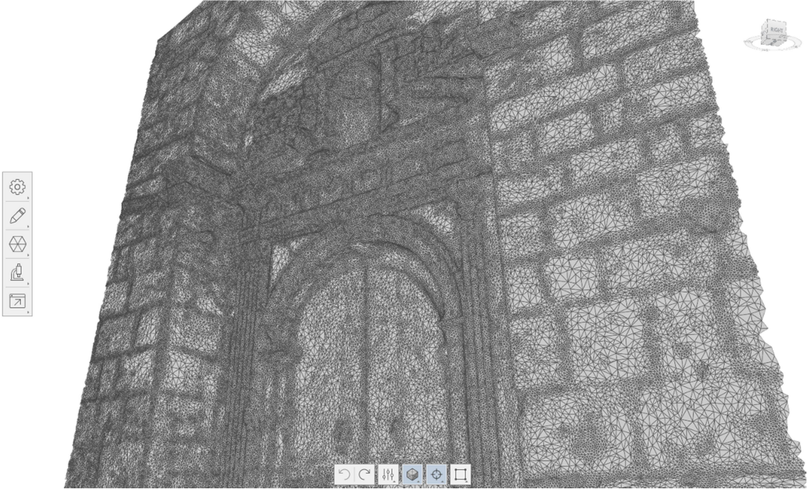
Figure 26. Model of meshing retrieved with Recap Photo.
