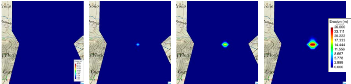
Figure 74. Smooth contour fill representation of the erosion. From left to right, erosion at times 1200 s, 2400 s, 3600 s and 4800 s.
