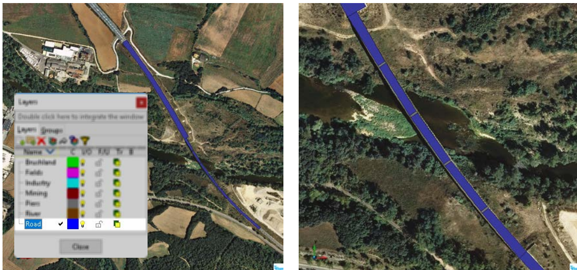
Figure 50. Representation of the “Road” geometry. On the right side we can observe how the new layer (“Road”) has been joined with the existing one (“Piers”).
