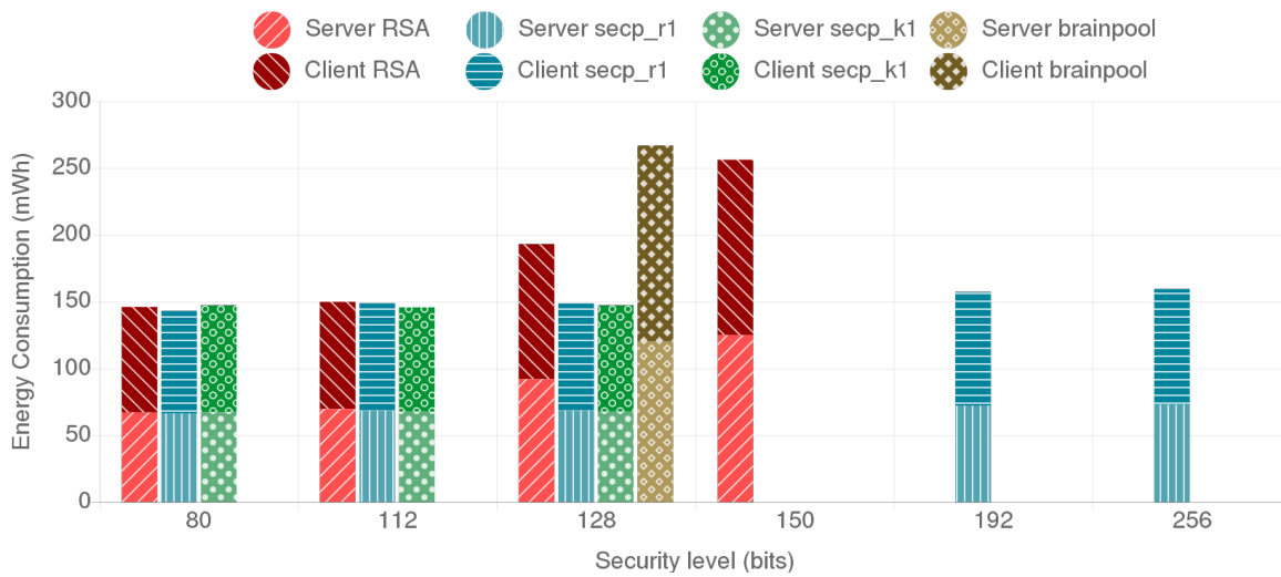
Figure 9. Mist end-device server and mist end-device client combined energy consumption for the different tested alternatives.
