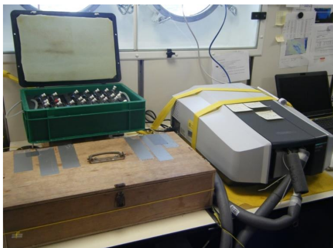
Figure 11. Spectrophotometer on the right, the wooden box is the incubator and above it, the cells for pH measurements as they were set up in the Trokenlabor at the R/V Maria S. Merian. Photo taken by N. Fajar.
