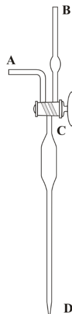
Figure 14. Equipment for TA determinations. On the computer's right in order, Titrande 904 , stirrer 801 (Metrohm) and knudsen pipette attached to an air pump. On the right, schematic Knudsen pipette , which allows quick and accurate transfer of a constant volume of liquid (sea water). A double sided vent (C) allows for either the establishment of a flow between the body of the pipette and one of the branches (A or B) or the isolation of the body from both branches.
