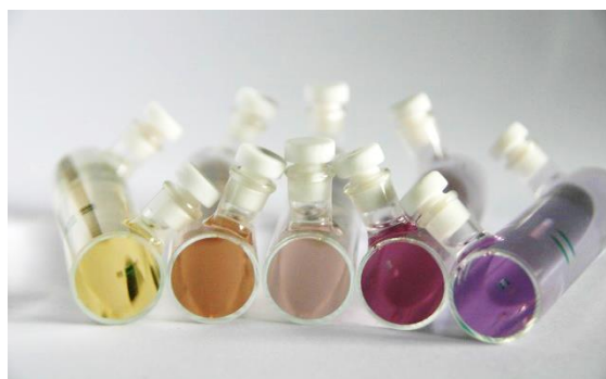
Figure 10. Cylindrical cuvettes for pH determinations. Made of quartz they can also be used for carbonate ion determinations. On the right, the range of colours of m -CP from the single protonated form to the fully deprotonated species.
