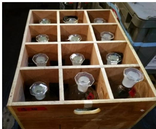
Figure 13. Box for transporting TA sample bottles from laboratory to sampling area and viceversa.
