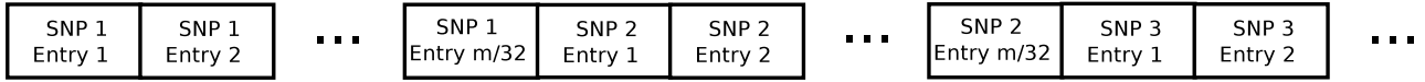
Fig. 7. Example of one array with the information of one SNP without reordering the entries.
